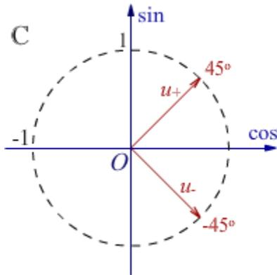
The figure on the left shows two eigenvectors of rotation in a complex plane. The vertices of both are located on a unit circle with the center at the origin. The first ( $u_+$ ) is the angle  $\frac{\pi}{4}$  radians ( $45^\circ$ ) with the abscissa, and the second  $-\frac{\pi}{4}$ . Another way to write the same is:
